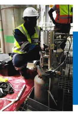
Pressure safety valves installed on industrial plant protect life of employees and avoid damages on equipment in case of excessive pressure. A periodic calibration is one of the most important requirements to ensure that the safety valves will provide this critical protection.
