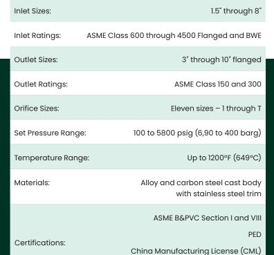
The 1700 Series Maxiflow high-pressure safety valve is a premium product that is installed on a majority of power generating stations worldwide to help protect boilers from overpressure conditions.
